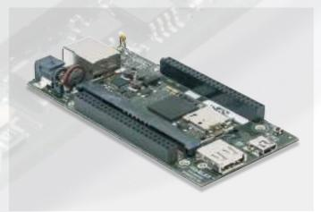
The IGEP<sup>™</sup> AQUILA EXPANSION is a fully equipped baseboard that access to all IGEP<sup>™</sup> COM AQUILA functionalities. It has been designed to be used as a reliable test and development platform and it can be used as the fastest way to develop and check the user's final application before building a prototype, saving costs and reducing time-to-market.
