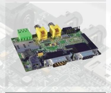
This expansion board has been designed to be used as a test and development complementary platform of IGEP<sup>™</sup> v2 DM3730. It can be used to check the final application in pre-prototyping phase, saving costs and reducing time-to-market.
