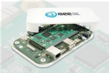
The expansion board is a fully equipped baseboard that access to almost all IGEP<sup>™</sup> SMARC<sup>™</sup> AM335x functionalities. It has been designed to be used as the fastest way to develop and check the user's final application before building a prototype, saving costs and reducing time to market. This model can be used with all the IGEP<sup>™</sup> SMARC<sup>™</sup> series modules.
